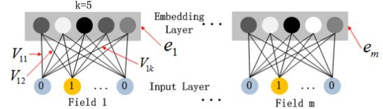
Figure 4: The structure of the embedding layer
