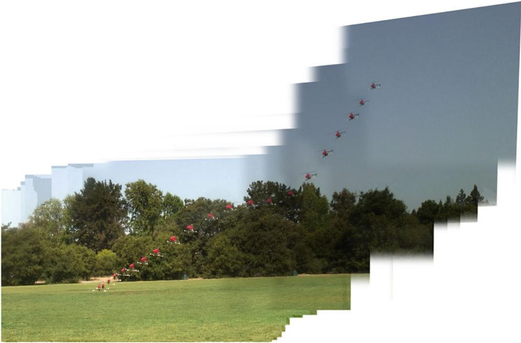
**Autonomous Helicopter Flight Using Reinforcement Learning, Fig. 4** Superimposed sequence of images of autonomous autorotation landings (from Abbeel et al. 2008)
