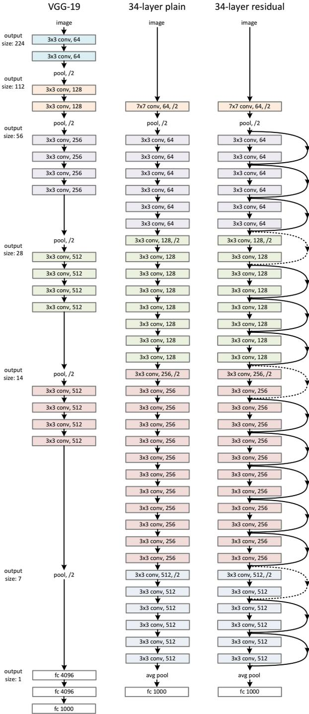
Figure 3. Example network architectures for ImageNet. **Left:** the VGG-19 model [41] (19.6 billion FLOPs) as a reference. **Middle:** a plain network with 34 parameter layers (3.6 billion FLOPs). **Right:** a residual network with 34 parameter layers (3.6 billion FLOPs). The dotted shortcuts increase dimensions. **Table 1** shows more details and other variants.
