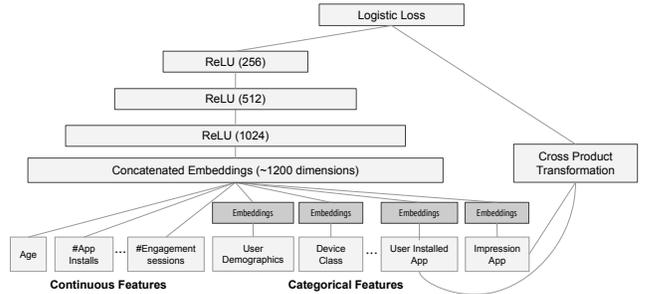
Figure 4: Wide & Deep model structure for apps recommendation.
